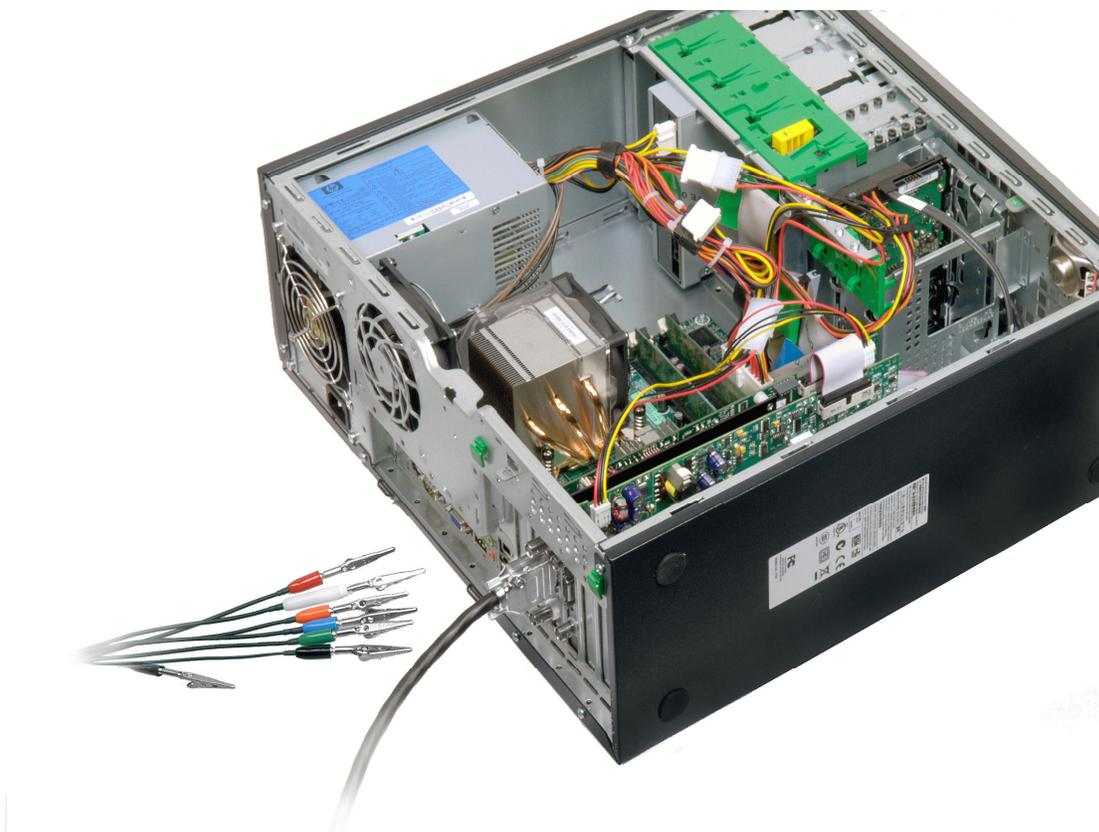
**Installed Potentiostat with Cell Cable Attached**
